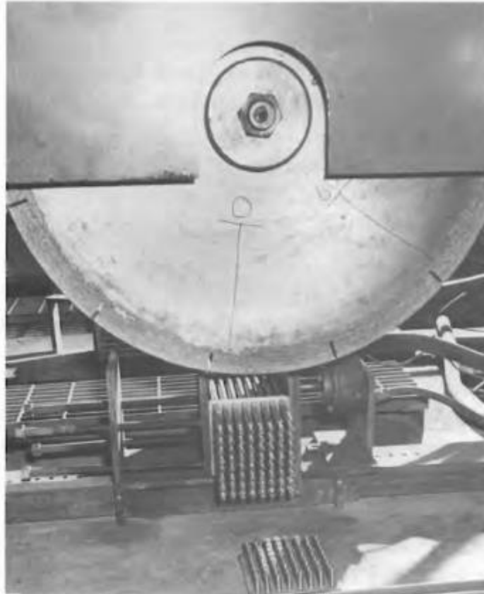
Simulated BWR Fuel Bundles with Springs Shown as Cut on the PNL Arc Saw
